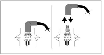
Figure 26. Disconnecting/Connecting Spark Plug
